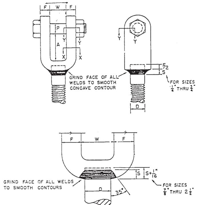
FIG. 6 Arc or Gas Welded-Jaw End Pull
