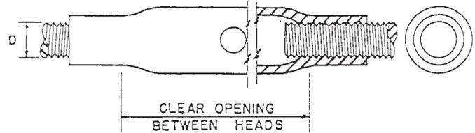
FIG. 13 Type II, Pipe Turnbuckle Body
