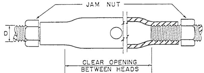
FIG. 14 Type III, Rigging Turnbuckle Body
