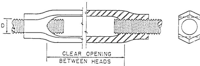
FIG. 10 Type I, Grade 2, Open Turnbuckle Body, Spread
