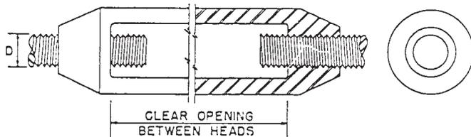
FIG. 9 Type I, Grade 1, Open Turnbuckle Body, Forged
