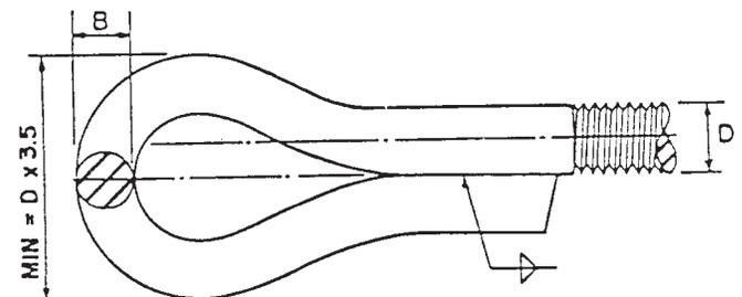
FIG. 4 Arc or Gas Welded-Eye End Pull
